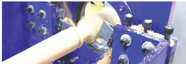
Carbide Lathe Knife Hardness:91-91.5 HRC
