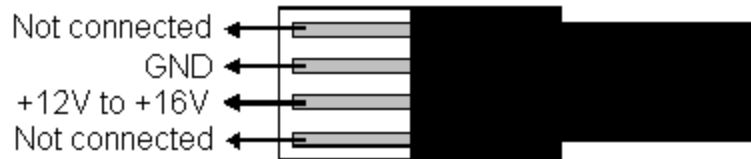
FIG. 1-7 MOLEX CONNECTOR PIN-OUT IN BT VERSION
