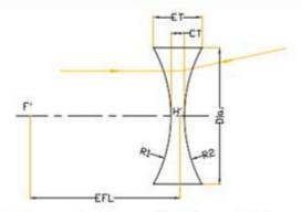
UM offers various specifications of biconcave lens. The biconcave lens has a negative focal length, which gives it a wide range of applications. They are used for image reduction and to spread light.
