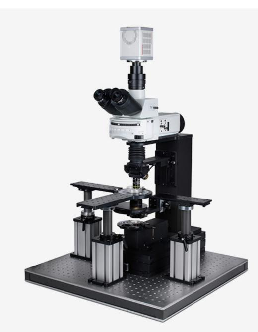
uM-Scope for dual patch clamp and wide field fluorescence imaging: XYZ-motorized microscope, transmitted light illumination, dual uMp-3 manipulator system and rigid posts for the manipulator and sample mounting:
