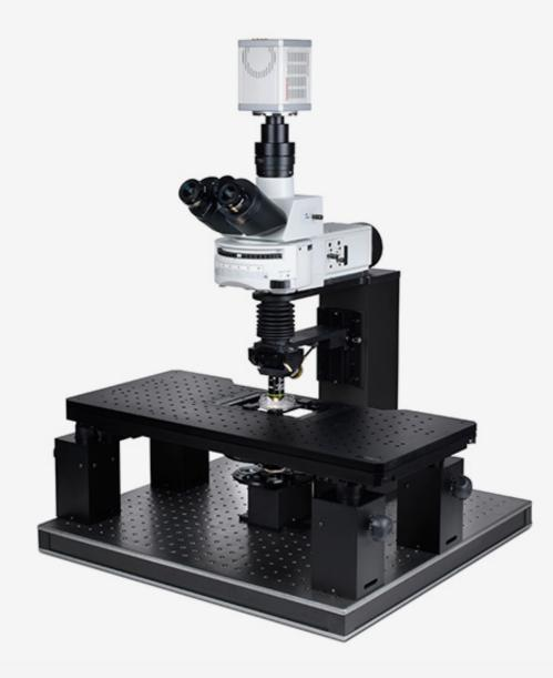
uM-Scope for 4-channel in vitro patch clamp experiments: motorized focus, motorized xy-stage, transmitted light illumination and quad uMp-3 manipulator system:
