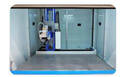
The combined motion of the XYZ axes covers an area of 1,000x500x500mm, and the steel structure guarantees the stability and rigidity of the entire system.
