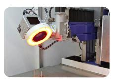
This laser marker is set up for **integration** with several accessories, like the rotating head. Additionally, it can be equipped with a 3-axis-head to mark cylindrical parts, with a
