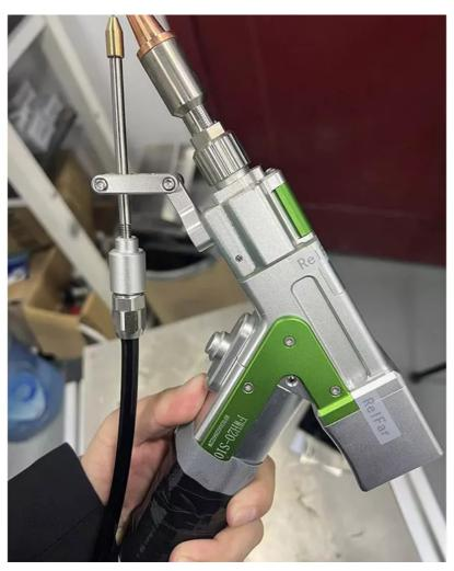
The hand-held laser head is simple in appearance, small and light, and can be used by hand for a long time. The integrated design of buttons and handles is simple and easy to use. The built-in scanning system adopts a small high-speed motor and drive. The main body is integrally processed and formed, which is sturdy and dust-proof, stable and durable. It can be switched between cleaning and cutting according to different scenarios, which is convenient and easy to operate.
