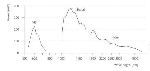
Typical power vs. wavelength chart, measured with a OPO-X / taccor tune laser.
