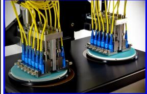
Scepter workholders feature Independent Suspension (IS) at each connector position for controlled pressure and uniform contact with the polishing surface. IS permits air polishing while maximizing film life. Each position is optically aligned for optimal polish geometry using KrellTech's patented technology.
