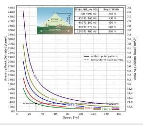
Example: VUX- $160^{23}$  at 600,000 pulses/sec, laser power level 100% altitude 1,300 ft AGL, speed 30 kn, resulting point density  $\sim 34$  pts/m<sup>2</sup>
