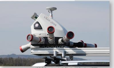
VMX-2HA equipped with 7 ball-joint directional RIEGL cameras
