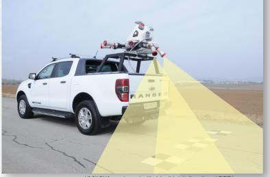
VMX-2HA equipped with 6 ball-joint directional RIEGL cameras, two ball-joint pavement cameras with close to NADIR orientation
