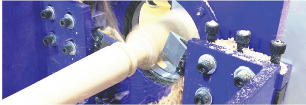
Carbide Lathe Knife Hardness:91-91.5 HRC
