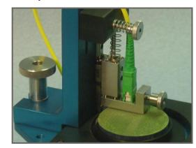
Proton™ workholders feature Independent Suspension (IS) for controlled pressure and uniform contact with the polishing surface. The workholder is also optically aligned. for optimal polish
