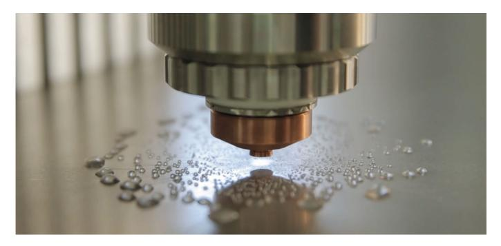
CoolTec: Ideal for permanent stable cutting of thick mild steel - due to direct water cooling of the sheet.
