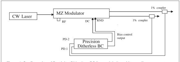
Figure 1. Configuration of Precision Ditherless BC for modulation with complimentary outputs
