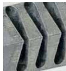
Microprocessing of co-balt-based carbide 200 \mu\text{m}
