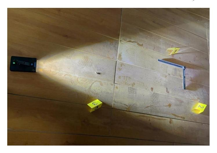
The OR-GZJ50 is a tough, lightweight and pocket construction crime scene light, specialized design for providing linear light illumination to identify and recover traces, tire prints, shoe prints evidence.
