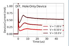
A space-charge effect leads to a current overshoot. Therefore, this technique is also called transient space-charge-limited current (T-SCLC) in literature. The time of the current overshoot is related to a transit time and allows the estimation of the charge carrier mobility and its field dependence. The occurrence of the current overshoot is a confirmation of good electrical contact for charge injection.
