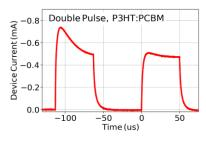
Double transient photocurrent pulses with varied delay times to analyze traps
