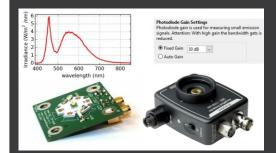
SOLAR CELLS: the main hardware is equipped with a suitable LED illumination system. A multi-LED board can be employed for External Quantum Efficiency (EQE) measurements.
