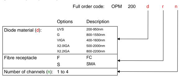
For example, a 2 channel, FC receptacle unit with a silicon (Si) photodiode input would be ordered as:
