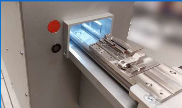
Fixture plate designed to hold 40 wires at 40AWG
