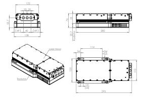
MPL2310 series laser head dimensions (in mm)
