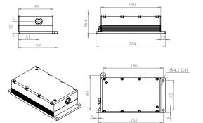
MPL2310 series laser head dimensions OEM version (in mm)
