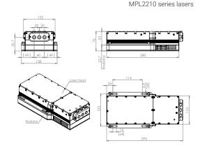
MPL2210 series laser head dimensions (in mm)
