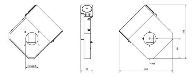
The MID14-24C diaphragm is compatible with standard 60mm Cage System.
