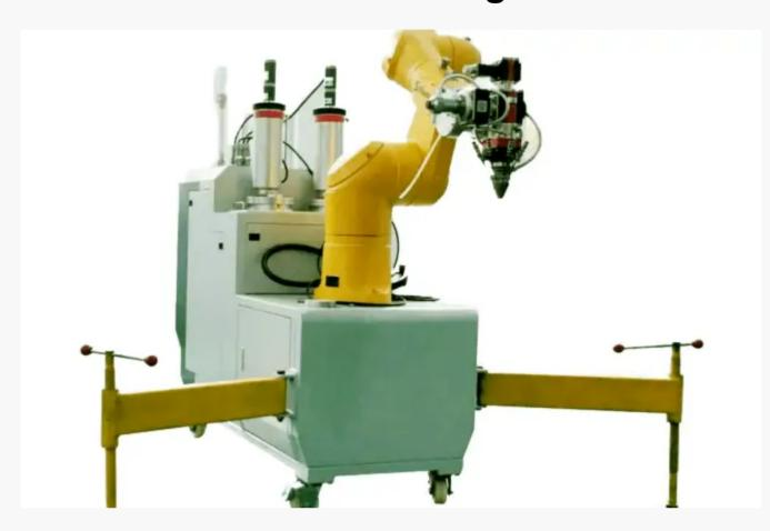
WALDUN's second generation of mobile laser cladding equipment can quickly integrate individual modules for repair work, saving customers downtime costs, disassembly costs and transportation costs for large equipment.
