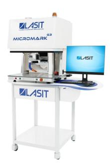
MicroMark G3 is a **compact**, functional bench **laser marker** that is able to meet the most varied production requirements while maintaining relatively low prices. The system is designed to also work with a robot thanks to the electric port. The machine is able to work independently by managing the door opening/closing times through the software.
