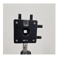
The MD12 is client-inspired very handy manually adjustable mechanical diaphragm. Intuitively simple aperture control consists of 4 independently-controlled aluminum sliding jaws, which can form either rectangle or square aperture of any size within 0...12mm range. Black anodized finish aluminum blades greatly reduce unwanted reflections. The MD12C model is adopted for implementation to standard 60 mm cage systems.
