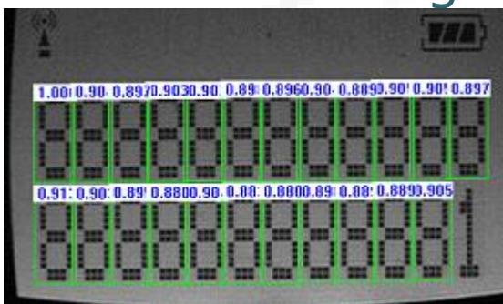
Pattern matching, also called template matching, is an excellent approach to locate known objects in an image. It works by providing a sample image of the item to be located and then searching for similar shapes in the target image.
