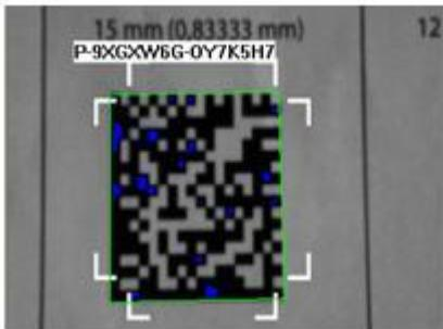
Another alternative to printed characters appeared more recently and is known as dot codes or 2D codes. They encode more information in the same space by allowing variations in two dimensions rather than one. To ensure data integrity, they also embed error detection and correction mean.
