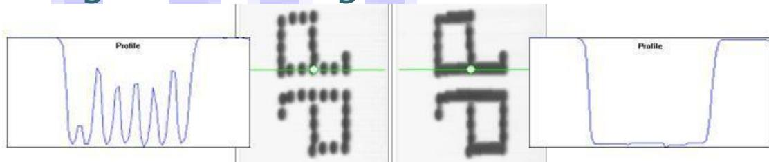
The processing functions are used to prepare the image by reducing unwanted nuisances such as noise or blur, or enhance some properties such as connexity of characters, contrast... They usually turn images into other images.
