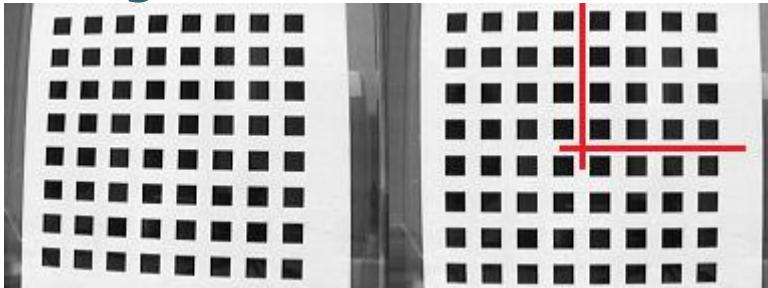
An image is said to be calibrated when a mapping correspondence has been established between the pixel coordinates and some real-world coordinates system established on the observe surface.
