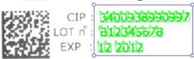
Many industrial applications require part identification. One of the ways to distinguish object is by printing a human-readable serial number on the surface or on a stickled label.
