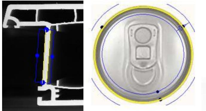
This function set is specialized in profile analysis (peaks in a 1D signal) and fitting of straight or circular lines. It puts emphasis in robust selection of the relevant edge points.
