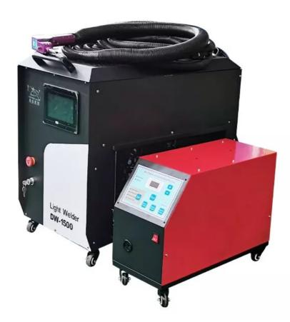
The clearly marked rear connection allows quick and easy entry. The laser transmission, gas and spray gun control are pre-connected to the 5 m (optional 10 m) cable. Simply plug in the power cord and gas connection, fix the cord clamp to the work surface and start using it. It can be connected to the network for fine-tuning and save the advanced parameter settings such as process parameters
