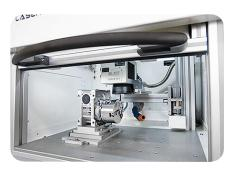
The **W** axis is available in various fixed or tilting versions, with different resolutions and holes for the passage of the bar. The axis is built with a preloaded crown gear and worm gear reducer, in order to have practically zero radial play. The motor has an integrated encoder and is controlled by FlyCAD.
