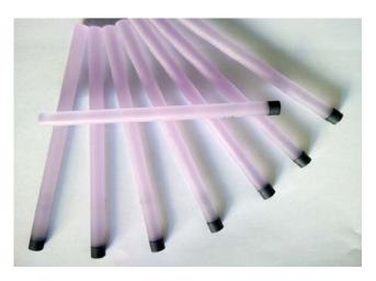
inorganic bonding aid. This innovative technology reduces thermal lens effect of laser crystals, provides integral components to make compact lasers.
