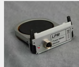
Laser power meter module (LPM) as insert in cover slide cartridge receptacle
