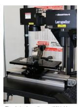
The photo shows the new X/Y table up close and integrated with a Langolier Open Table system.
