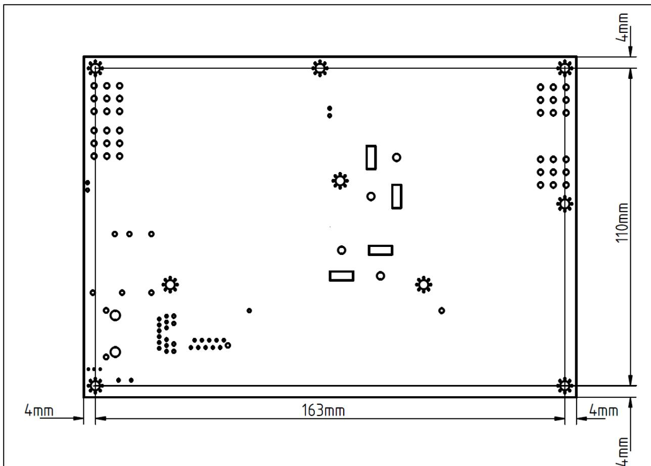
Mounting holes in the corner are 3.2 mm holes for M3 screws.
