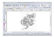
The Cutting Composer allows a wide selection of Vector formats to be imported or sent directly into Ethos form Corel Draw or Adobe Illustrator. Alternatively vector files can be created in the software using the many automatic drawing tools available. Access is also allowed to any True Type fonts that are loaded.
