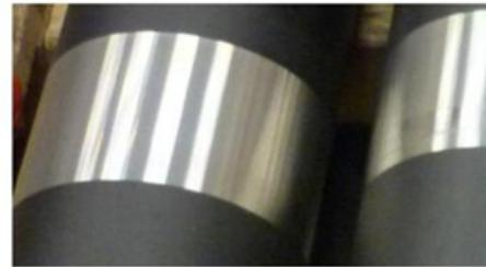
Steel pipe paint removal
