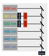
L6Cc and L4Cc integrate the largest panel of wavelengths from 375 up to 1064 nm combined in one channel or two independent channels.
