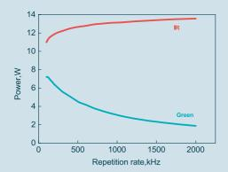
Average power dependence on the pulse repetition rate for infrared and green (SH) output
