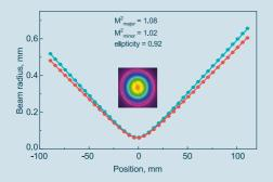
Beam quality measurement and beam profile in far field
