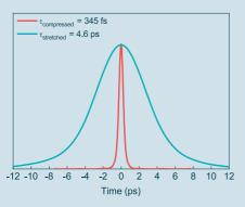
Pulse autocorrelation traces of compressed and maximally stretched 100 µJ pulses
