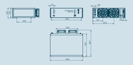
Drawing of Indylit 10 laser control unit (in mm)
