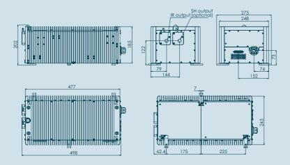
Drawing of Indylit 10 laser head (in mm)
