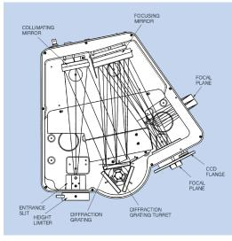
spectrograph. The imaging quality over the entire flat field has been maximized by using an asymmetric layout and a patented on-axis grating drive, reducing coma and other aberrations. A larger focus mirror allows the entire flat field to be used without vignetting (no throughput reduction at the edges of the focal plane).
