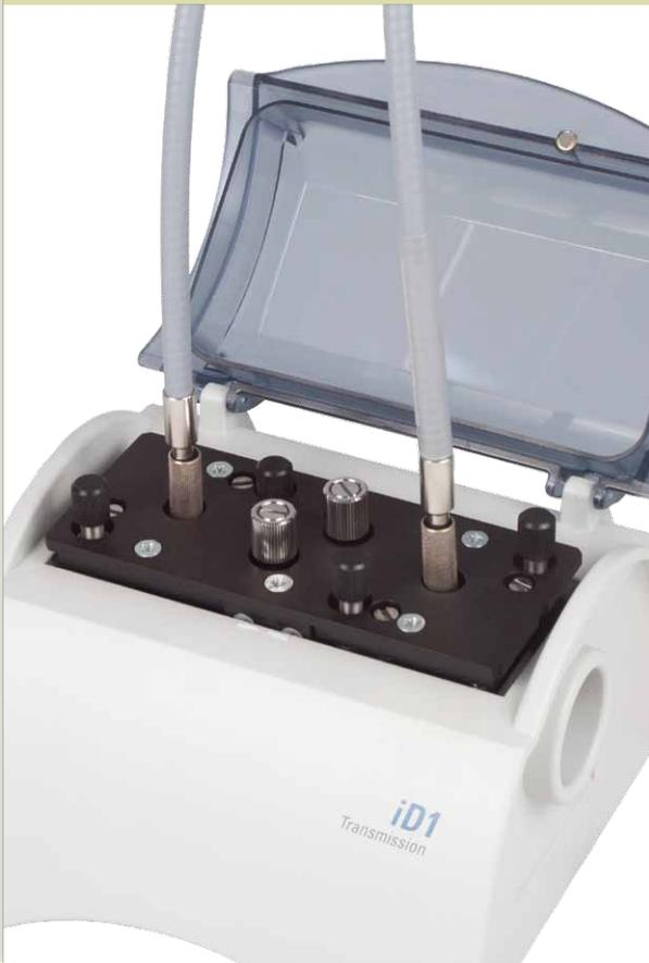
Fiber coupler FPC-2M enables efficient coupling of fiber probes with iS5 – the smallest FTIR-spectrometer from Thermo. FPC-2M design is based on two off-axis parabolic mirrors inside the standard accessories iD1 which can be adjusted for maximum signal from SMA-terminated probe.
