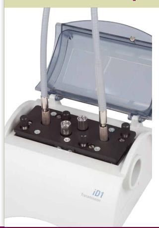
Fiber coupler FPC-2M enables efficient coupling of fiber probes with iS5 – the smallest FTIR-spectrometer from Thermo. FPC-2M design is based on two off-axe parabolic mirrors inside the standard accessories iD1 which can be adjusted for maximum signal from SMA-terminated probe.
