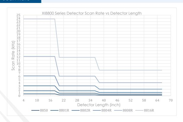
Calculate conveyor speed or object velocity by multiplying (Resolution \* Scan Rate) Example XI8804 16 inches long, Maximum velocity is (0.4mm \* 6kHz )= 2.4m/s
