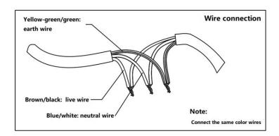
Connect the wires of the lamp to the electricity wire, and ensure that the colors of the connecting wires are the same (please refer to the detailed diagram). After the connection is completed, the waterproof and pull-proof treatment is required.
