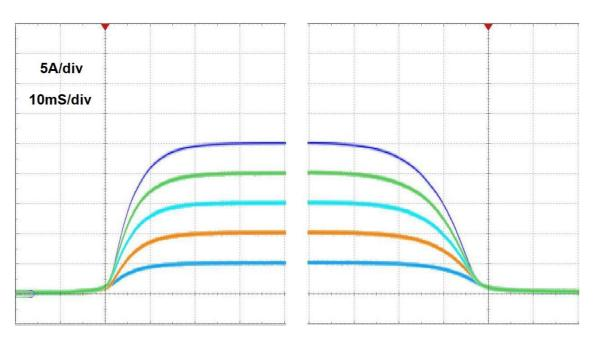
Figure 1. Typical current rise/fall time for Mode 1
