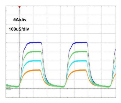
Figure 2. Typical current pulses fore Mode 2, triggering by F = 3kHz, Tp =  $150\mu s$
