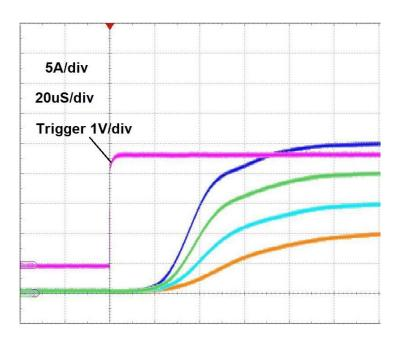
Figure 3. Typical trigger to current delay for Mode 2
