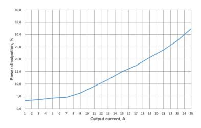
Figure 7. Power dissipation vs. output current at Vin=48V, Vout=30V
