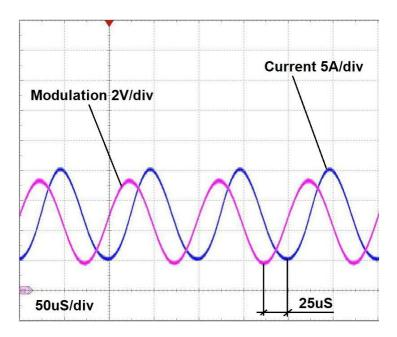
Figure 4. Typical current for Mode 3, analog modulation by sinusoidal 10kHz.
