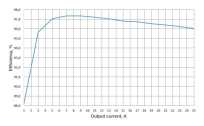
Figure 6. Efficiency vs. output current at Vin=48V, Vout=30V
