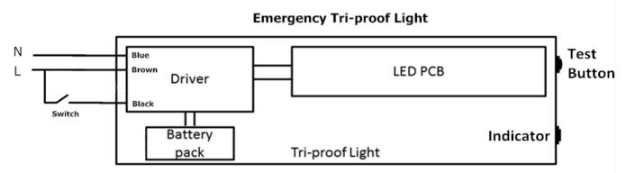
Customer can add a switch between Brown wire and black wire When switch on, the standard light will turn on, when switch off, the standard light will turn off
