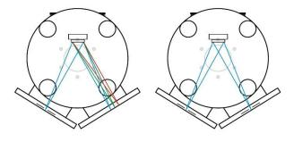
Operation modes: (1) Spectrograph, (2) scanning monochromator.
