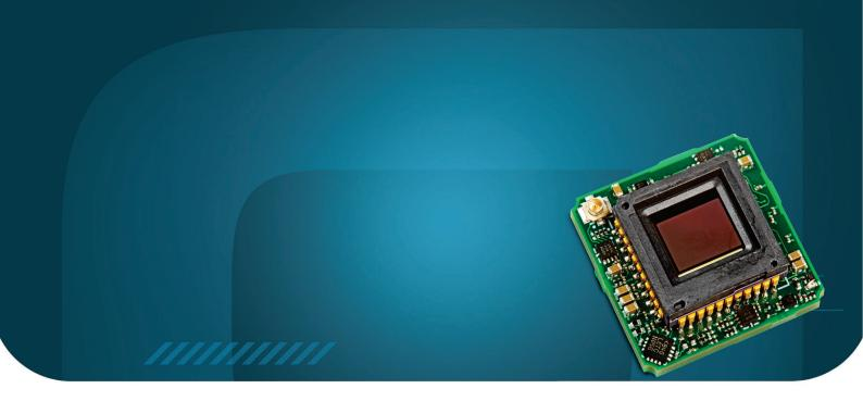
STATE-OF-THE-ART THERMAL IMAGING CORE
