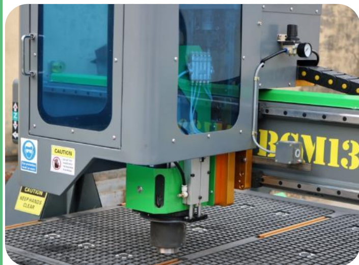
Italian HSD 9.5KW(12HP) Electrospindle with 10-position Automatic Tool Changer(ISO30)
