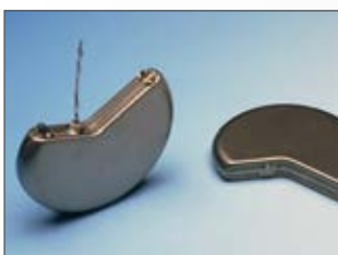
Laser seam welding pacemakers
