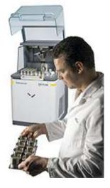
Zetium - Trace element analysis of geological materials using Zetium and Pro-Trace
