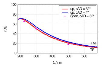
Typical efficiency curves based on rigorous electromagnetic modeling using measured AFM profiles. rDE refers to the ratio between diffracted power from the grating and reflected power from a mirror coated with the same material.
