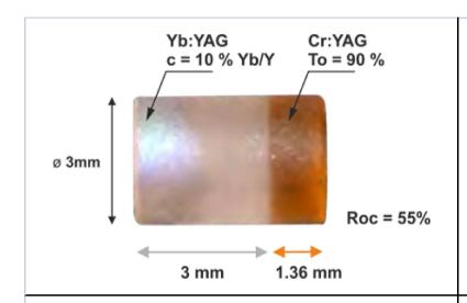
The Yb:YAG/Cr:YAG microchip laser threshold pumping power was found to be 3.3 W. With the increasing pumping power the mean output power, and generated pulse repetition rate also increased up to 1 W and 13.6 kHz, respectively, for the pumping power 9.3 W. The maxim output power was reached without observable thermal roll-over.
